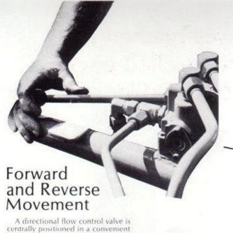
A directional flow control valve is centrally positioned in a convenient location giving forward and reverse movements as marked on a quadrant, from neutral to the selected direction.
